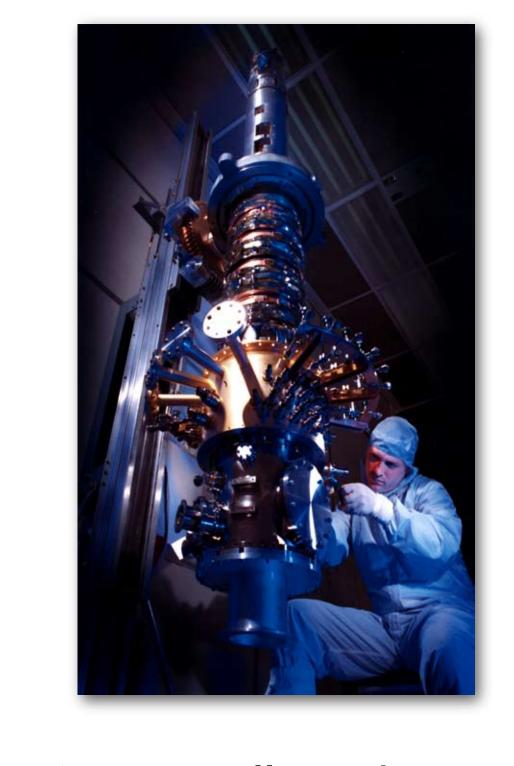
GP-B's 650-gallon dewar kept the science instrument inside the probe at a cryogenic temperature (2.3K) for 17.3 months and also provided the thruster propellant for precision attitude and translation control.
